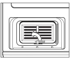
Turn the lever on the condenser unit to the vertical position.
